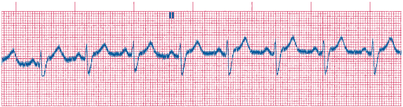
Fig. 17-6 A sinus rhythm tracing with 60-cycle interference. The baseline looks thick and fuzzy. The QRS is frequently not affected because of its greater height. Because 60-cycle interference has a continuous, consistent effect, the underlying rhythm can often be identified.
